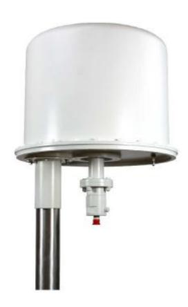
omnidirectional antennas ideally suited for command destruct / range safety applications. MSC high power omnis are rugged; radome covered, and can be tuned over a broad frequency range. The omni antennas are available in RHCP or LHCP and hemispherical or "donut" patterns. MSC's standard interface is 1-5/8" or 3 1/8". Type N, LC, and 7/8" EIA interfaces are also available depending on power requirements. Pole or stud mounts are available as well as custom mounts per your specification.
